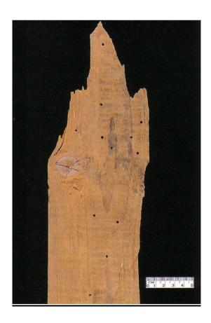
Softwood flooring revealing extensive Hadrobregmus Australiensis larval channeling. Note fungal growth on timber surface indicating conditions conducive to decay.
